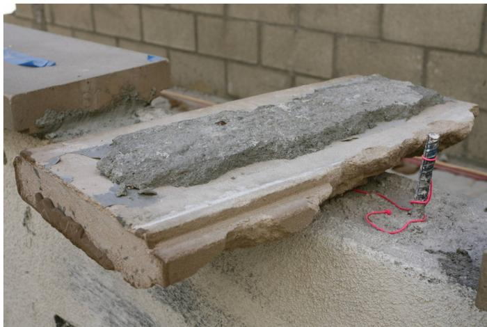
The added flexural bond was stronger than the precast concrete itself. Conventional polymer cement mortars had failed in bonding these cantilevered wall caps.
